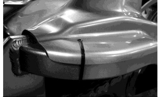
Position of cable tie
