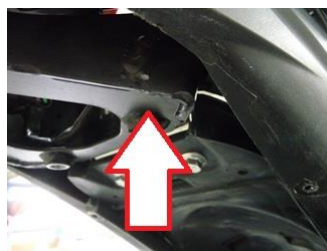
View of the pin removed
