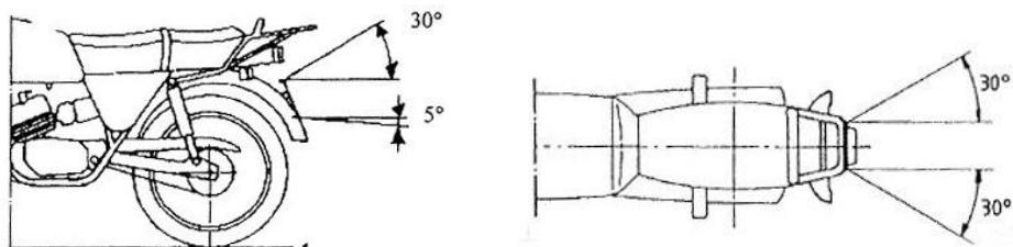
Width of number plate location: 280 mm - Height of location : 210 mm
