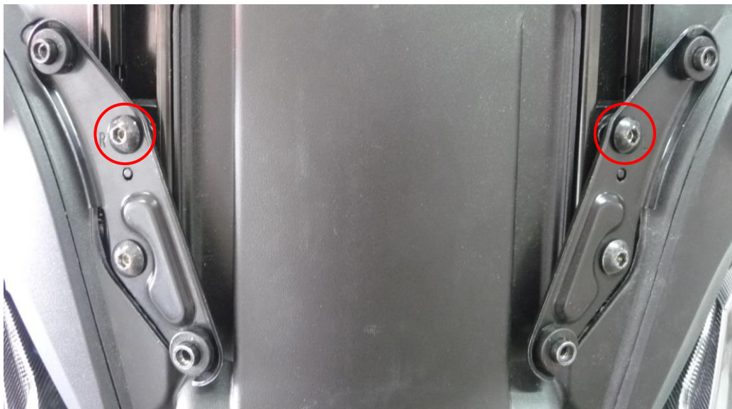
Screws to remove to insert the washer (it must be placed under the fixation)
