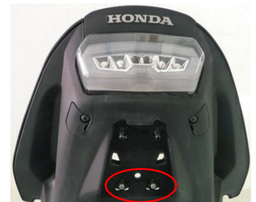
Fitting screws of the undertray
