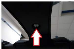
Phillips screw of the rear mudguard
